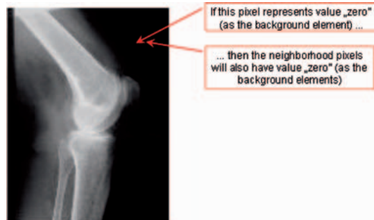
Fig. 3.6. The simplest method of lossless compression consists in the abbreviated coding of groups of pixels with the same grey level
