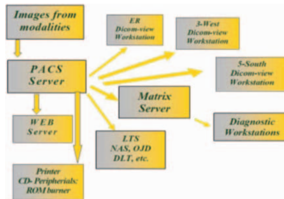
Fig. 3.4. The role of a PACS system as the distributor of medical images
