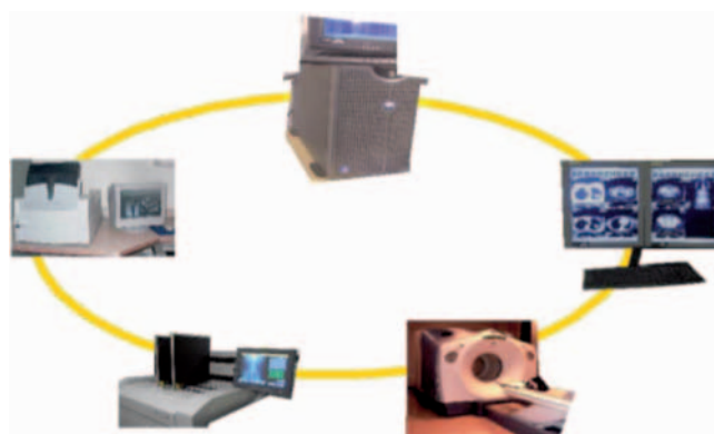
Fig. 3.1. An example structure of an older generation PACS system with a separate FDDI ring for fast image transfer (source Internet)
